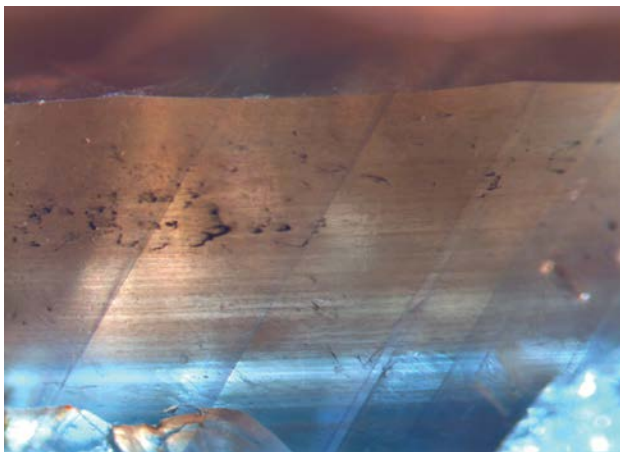
Figure 9: This view of the girdle of a Gold Sheen sapphire shows parallel brownish lines representing networks of needle and platelet inclusions along the basal pinacoid, and also a set of parallel lines (polysynthetic twin planes) oriented at about 58° and 32° to the basal pinacoid and the c-axis, respectively. Photomicrograph by T. N. Bui using darkfield illumination; magnified 30×, field of view 4.76 × 3.35 mm.
