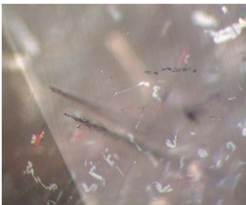
Figure 14: Needle-like inclusions consisting of diaspore and boehmite particles (appearing dark in brightfield illumination) lie along polysynthetic twin planes in the Gold Sheen sapphire. Photomicrograph by T. N. Bui; magnified 200×, field of view 360 × 300 μm.
