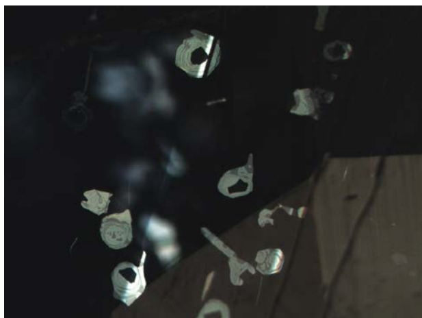
Figure 5: The platelets in this sapphire contain dark areas and appear to be composed of different minerals. Photomicrograph by T. N. Bui using brightfield illumination; magnified 50 \times , field of view 1.3 \times 1.0 mm.
